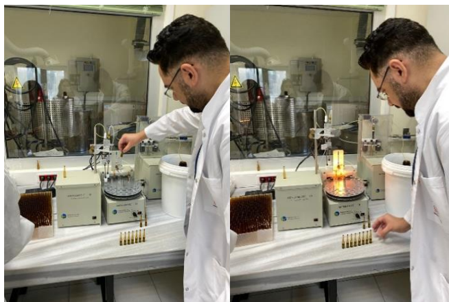
Figure 5. Bottling process of the UME CRM 1335.
