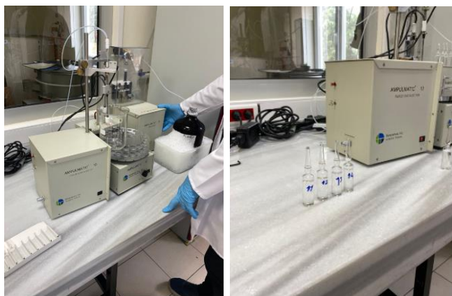
Figure 4. Bottling process of a primary standard of pure ethanol.
